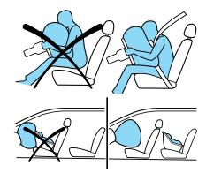
**WARNING:** All occupants of the vehicle, including the driver, should always properly wear their safety belts, even when an air bag supplemental restraint system (SRS) is provided.
